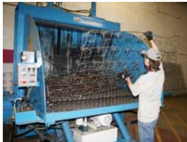
The invention of the Coil Spring Compactor by a Duluth inventor helped NRRI find markets to recycle the components of old mattresses. The business model is a proven success at Goodwill Industries.
